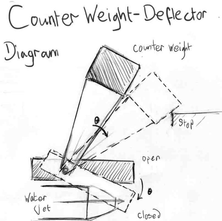
The problem with the past generators was that the shaft that holds both the counterweight and the deflector, was too small to support the counterweight (which not only moves back and forth in its plane of rotation but wobbles to the sides as well, causing extra unwanted stress).
