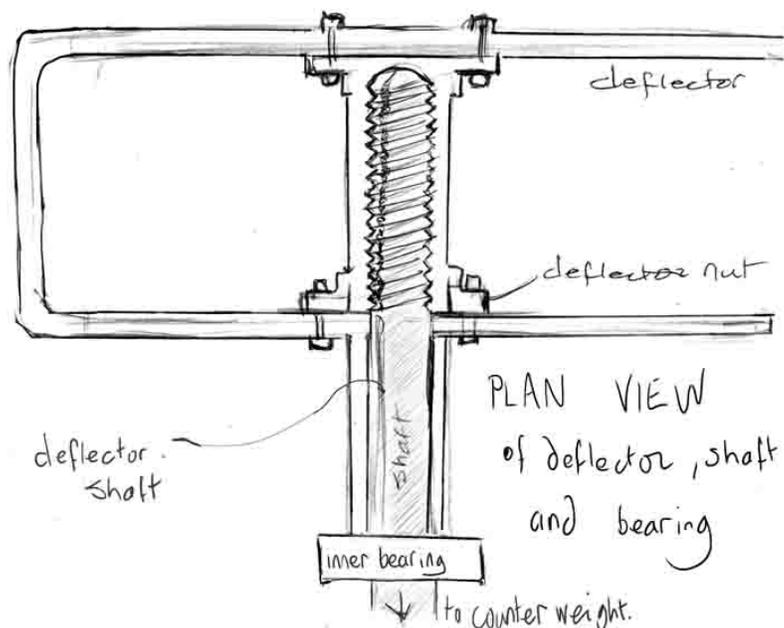
The threaded portion is either threaded left or threaded right, depending on which turbine it is located, as one turbine is the mirror image of the other. The idea behind this is that as the water exits the nozzle and hits the deflector, it will push the deflector in such a way that the deflector will want to rotate and either loosen or tighten the attached
