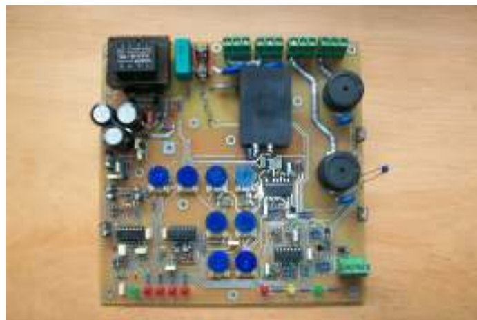
Hummingbird ELC with everything mounted on one board
